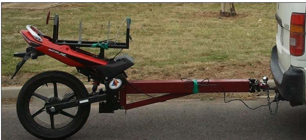
Figure 6-1: Conceptual illustration (top) and photograph (below) of the idealised physical quarter car (SWEV).
