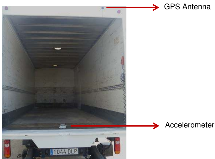
Figure 8-79: The location of the accelerometer and GPS antenna in the rear of the heavy truck.
