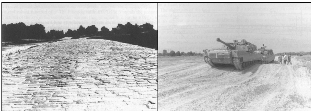
Figure 3-7: Photographs of the Belgian Block (left) and Perryman3 (right) courses, from Chaika et al. (2004).
