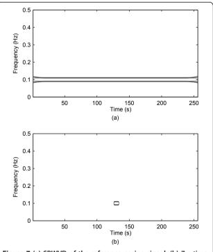
Figure 7 (a) SPWVD of the reference cosine signal; (b) 7 s time slice of the SPWVD around  $p=130~{\rm s}.$
