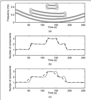
**Figure 9** (a) SPWVD of a three-component signal with parabolic FMs; (b) number of components in time ( $\alpha$  = 3 dashed,  $\alpha$  = 7 solid,  $\alpha$  = 11 dotted),  $\Delta t$  = 7 s; (c) number of components in time ( $\Delta t$  = 3 s dotted,  $\Delta t$  = 7 s solid,  $\Delta t$  = 23 s dashed),  $\alpha$  = 7.
