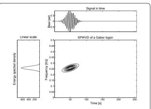
Figure 2 A Gabor logon in time (top), frequency (left), and joint time-frequency domain using the SPWVD (center).
