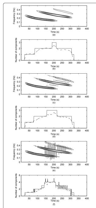
Figure 12 (a) SPWVD of a bat echo location signal; (b) number of components in time (thresholded results-solid line, results without thresholding-dashed line); (c) MBD of a bat echo location signal; (d) number of components in time (thresholded results-solid line, results without thresholding-dashed line); (e) CWD of a bat echo location signal; (f) number of components in time (thresholded results-solid line, results without thresholding-dashed line).
