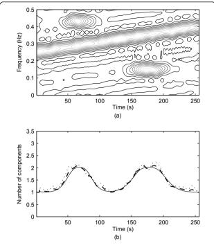
Figure 11 (a) SPWVD of a signal composed of an LFM component and two Gabor logons embedded in additive white noise with SNR = 10 dB; (b) number of components in time for the noise-free signal (solid), signal corrupted by additive white noise (SNR = 15 dB (dashed), and SNR = 10 dB (dotted)).
