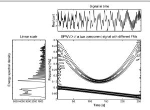
Figure 5 A two-component signal composed of a parabolic FM component and an LFM component, in time, frequency, and joint time-frequency domain (SPWVD).
