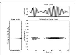
Figure 4 Two Gabor logons with different time durations, shown in time, frequency, and time-frequency (SPWVD).
