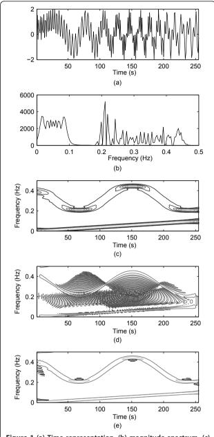
Figure 1 (a) Time representation, (b) magnitude spectrum, (c) spectrogram, (d) WVD, and (e) SPWVD of a two-component nonstationary signal.
