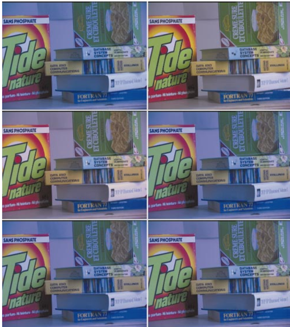
Fig. 9. Color correction of real images: Top left, original image; top right, target image; middle left, neural network estimate; middle right, gamut-mapping algorithm; bottom left, WP algorithm; bottom right, GW algorithm.
