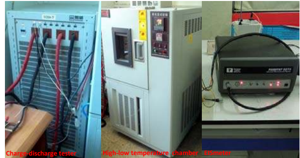
Fig. 3. Dedicated battery charge-discharge tester (left), thermally controlled environmental chamber (middle) and electrochemical impedance spectroscopy instrument (right).
