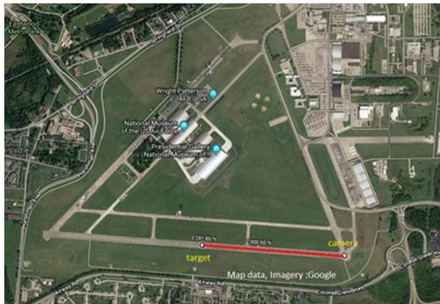
Fig. 3 The 1-km experimental path over the runway with camera and target locations shown.
