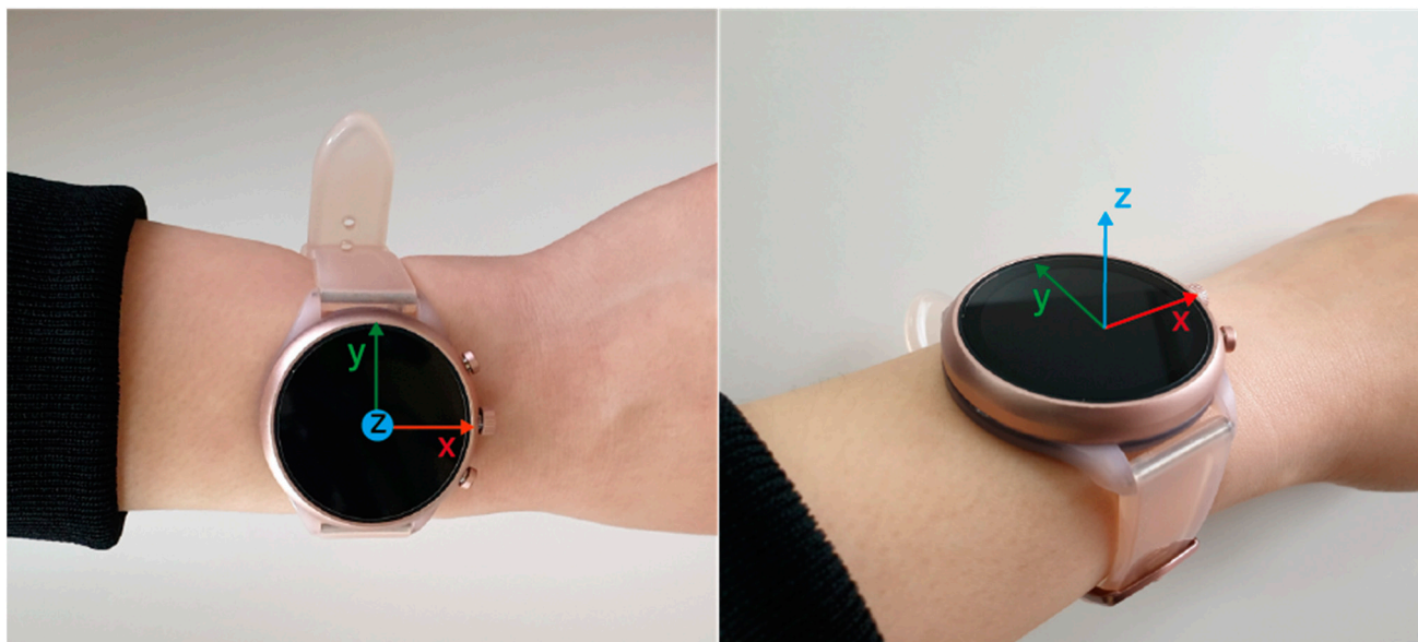
Figure 3. The smartwatch with its axis displayed adopted for the experiment.
