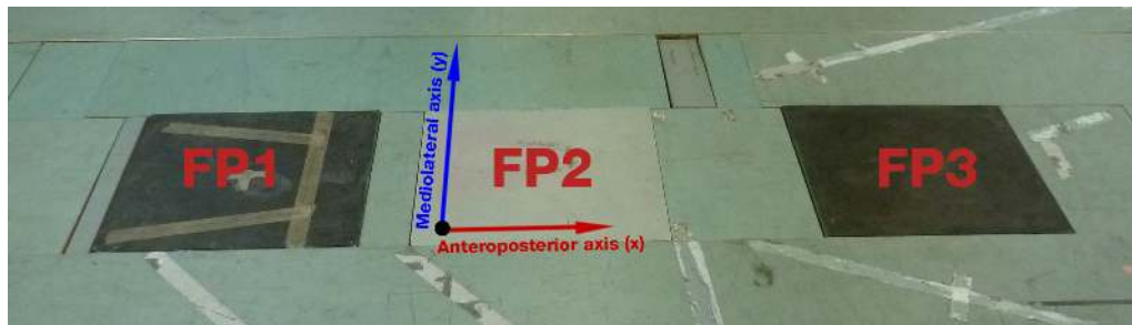
Figure 2. The three AMTI force plate system used, denoting the coordinate system of the laboratory. The vertical axis ( z ) points upwards, perpendicular to the anterior ( x ) and lateral ( y ) axes.
