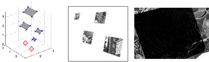
Figure 5: Bundle adjustment: (left) artificial setup for bundle adjustment, (middle) example image for one camera position; Homography estimation: (right) overlay of images using the homography estimated with covariances.
