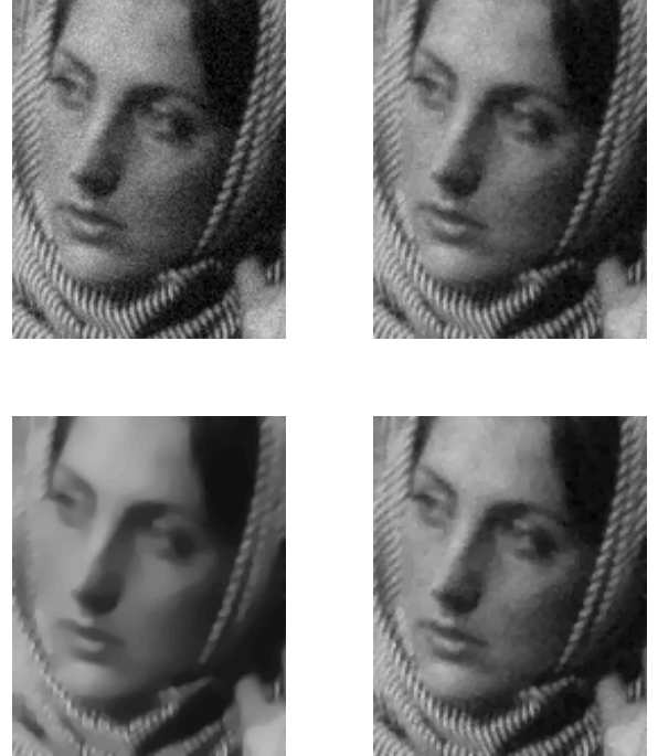
Fig. 13. Effects of stopping criterion on processing results of different stopping times, processing Barbara image (head part is shown). Top left: noisy image f ; Right - Weickert's method (24). Bottom left: Mrazek-Navara (23), right - our method of direct estimation.
