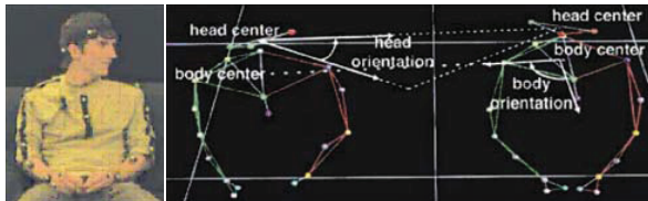
Fig. 2. MoCap markers and body/head orientation features.
