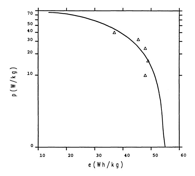
Figure 4. Power-energy plot for a  $Zn/Br_2$  battery.
