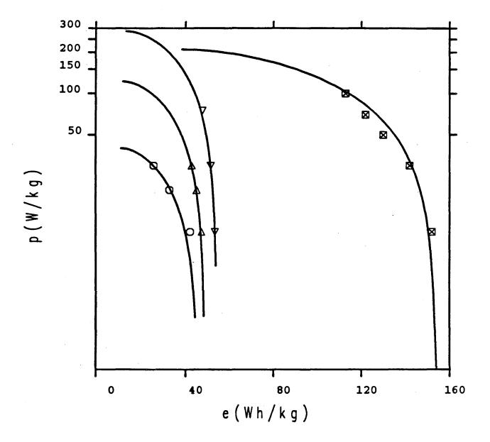
Figure 3. Power-energy plot for various secondary batteries. Eq. (5), parameters as listed in Table 2 Experimental data from references listed in Table 2 O Pb/PbO<sub>2</sub>, v = 12.0v Δ Fe/NiOOH, v = 6.0v ∇ Zn/NiOOH, v = 6.4v ⊠ Na/S, v = 1.85v
