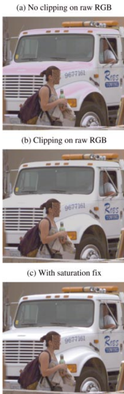
Fig. 1. Kodak DCS200 image rendered (a) without any saturation fix, (b) with pixel-value clipping to a known white point, and (c) with saturation fix for an image with a large number of saturated pixels. Pixels at the face areas of the images are scrambled to protect the privacy of the subjects.
