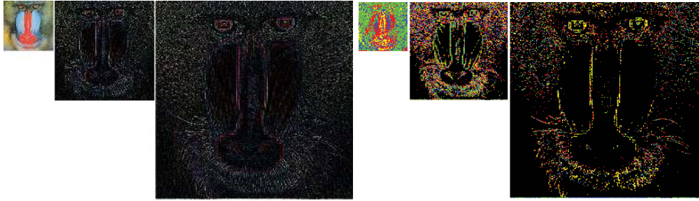
Fig. 5.7 A multiscale representation of the baboon image. Left: twice subsampled image and its residuals at two higher levels. Right: the segmentation of vectors ( 2 \times 2 blocks) by a hybrid linear model at each level—different subspaces are denoted by different colors. The black regions correspond to data vectors whose energy is below a given error threshold.
