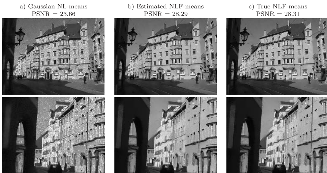
Figure 12. Denoising of a hybrid noise with true parameters (a, b, c) = (0.0312, 0.625, 100) , initial PSNR = 20.34dB. The noisy image is displayed on Fig. 5-a. a) Standard NL-means assuming and estimating Gaussian noise, b) NLF-means with the estimated NLF and c) NLF-means with the true NLF.
