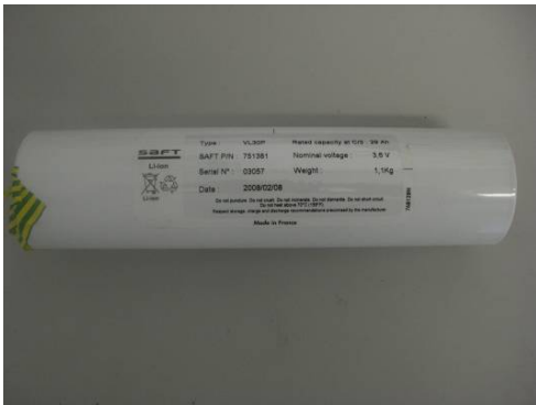
Figure 1: Lithium-ion VL30P cell from SAFT
