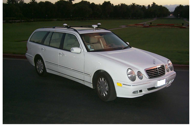
Fig. 3. Test Vehicle with Two-Antenna GPS Set-up
