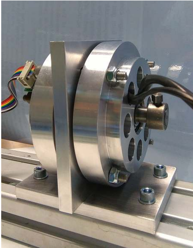
Figure 58: A Kollmorgen RBE type 12 pole frameless motor as used in the simple test setup. The aluminum casing was made to fit the motor and allow for testing to obtain the motor performance characteristics. The sensors in the motor include hall sensors for the commutation of the motor and an optical incremental encoder for the position of the motor. A small ring is clamped to the main axle to be able to turn the motor axle manually.
