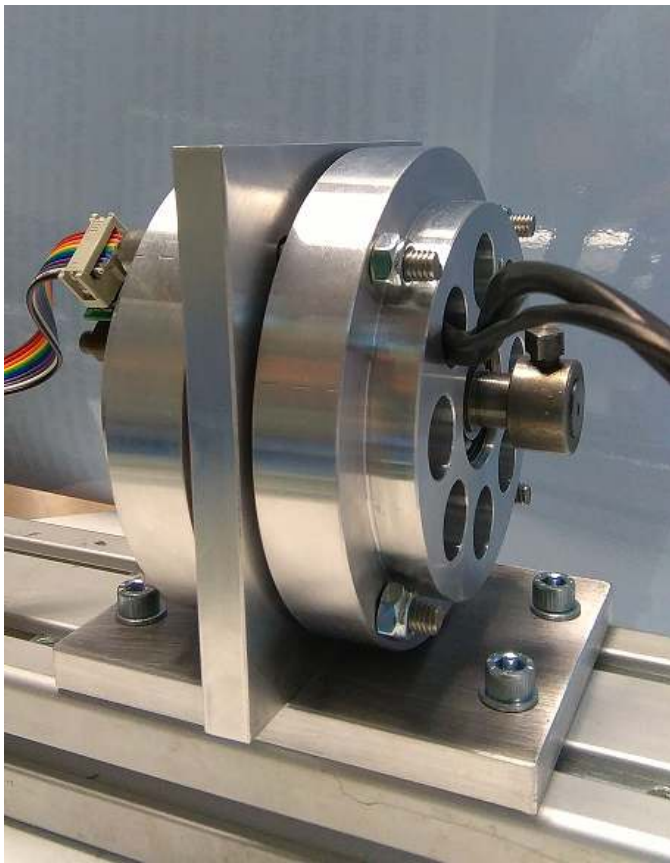
Figure 2. A Kollmorgen RBE type 12 pole frameless motor as used in the test setup. The sensors in the motor include hall sensors for the commutation of the motor and an optical incremental encoder for the position of the motor. A small ring is clamped to the main axle to be able to turn the motor axle manually.
