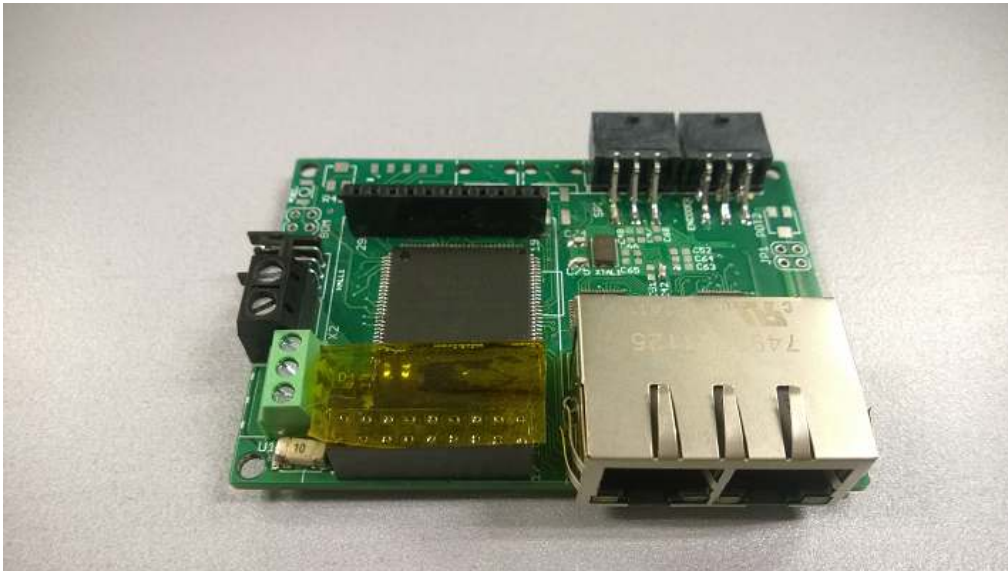
Figure 64: Exotronics Board produced by Victor Grosu [12]. This board can be used in combination with a motor drive like for example an Maxon ESCON. The board can read an incremental encoder, a magnetic (SPI) encoder, a loadcell and other IO. The board can send a pwm setpoint to the motor controller.
