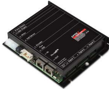
Figure 65: Maxon EPOS3 controller. The EPOS3 controller is a versatile motor drive that can be configured for position, velocity and torque control. These are no longer sold by Maxon. Alternatives are MAXPOS and EPOS4 drivers. These drives 'speak' EtherCAT and can easily be imported into TwinCAT. Extensive documentation on the devices can be found at the specific page on the website under downloads
