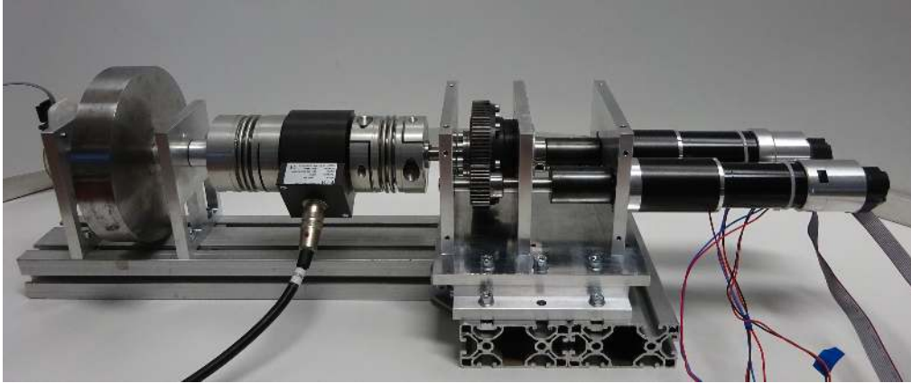
Figure 61: Dual-motor actuator setup. The setup consists of two DC motors coupled to the same output by means of a planetary differential. Holding brakes on the motors allow switching off the motor, while the brake delivers a static torque. The output is a simple flywheel. A speed controller for the setup, using information from the encoder on the output as feedback, is programmed in Simulink and run on the TwinCAT target at a speed of 1 kHz.
