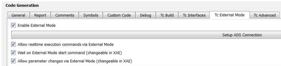
Figure 17: The ADS (Automation Device Specification) protocol is set up between MATLAB and TwinCAT. Check all boxes to allow the Simulink model running on the real-time target to be controlled by the Simulink model running on MATLAB.
