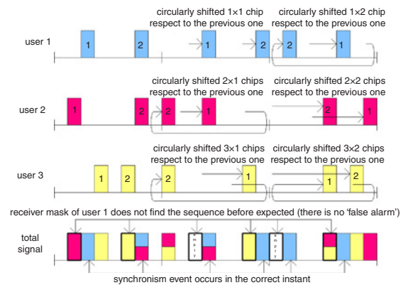
Fig. 1 Illustration of proposed circular shift mechanism and its efficiency to avoid 'false alarms' (example for s = 3 users, m = 3 synchronisation bits and code parameters L = 8 and w = 2 )
