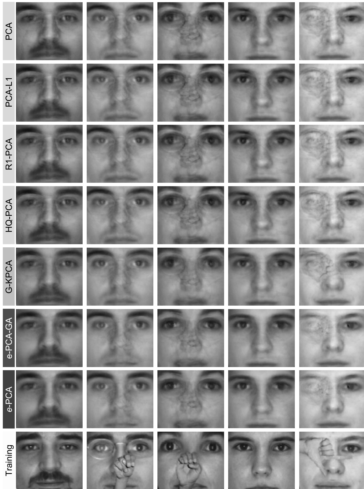
Fig. 12 Reconstructions of PCA, PCA-L1, R1-PCA, HQ-PCA, G-KPCA, e -PCA-GA and Euler-PCA (top to bottom) after learning with 50 % hand occluded images (20 components). The bottom row shows the training data. The uncorrupted images are shown in Fig. 3
