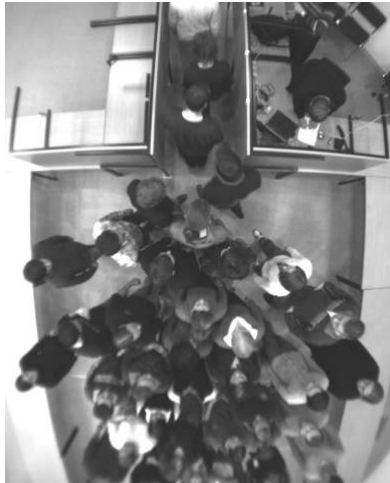
Fig. 1. Clogging near a bottleneck. The shape of the clog is discussed in more detail in Sec. 4.5.
