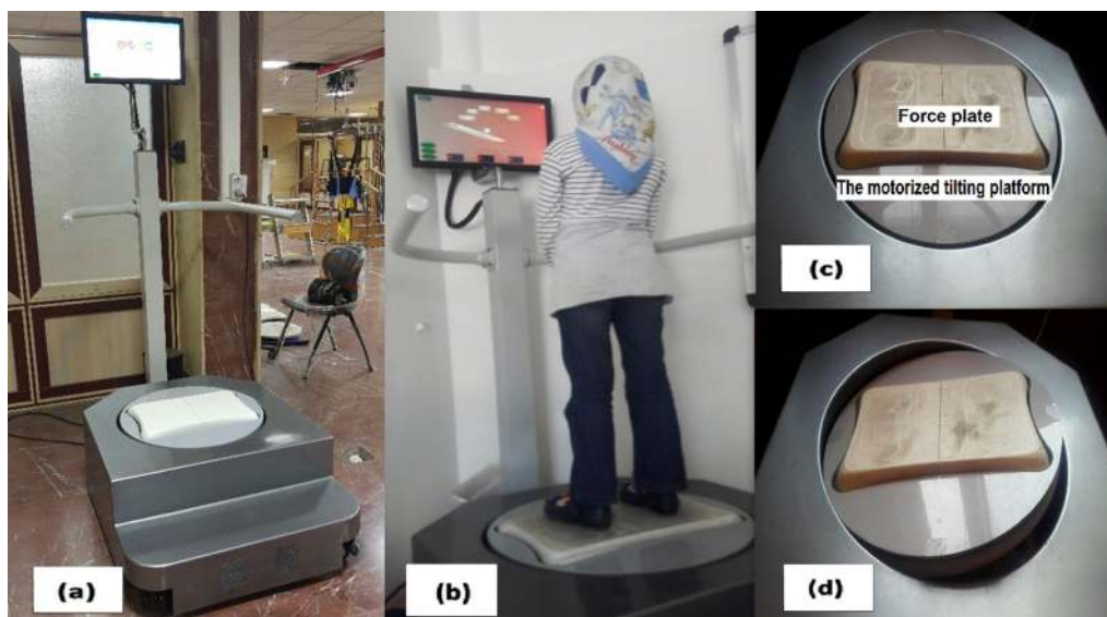
Fig. 2 A robotic device was adopted to implement the new VWM-B training program. a An overview of the robot, b The whole setup while the subject performs a training trial, c The motorized tilting platform and the force plate, d An example of the tilting function
