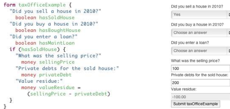
Figure 2: An example of a textual QL model (left) and its default rendering (right).
