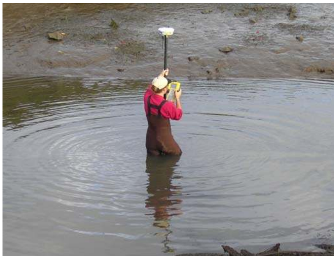
Recording GPS position of depth sensor.
