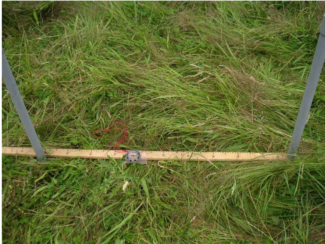
Figure 4.7. Sediment Accretion Stakes
