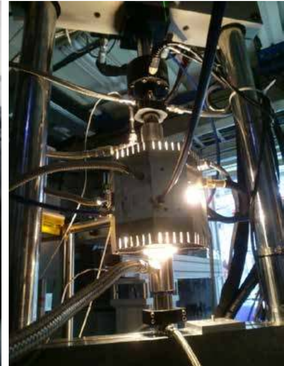
Assembling heater, grips and specimen at Argonne APS
