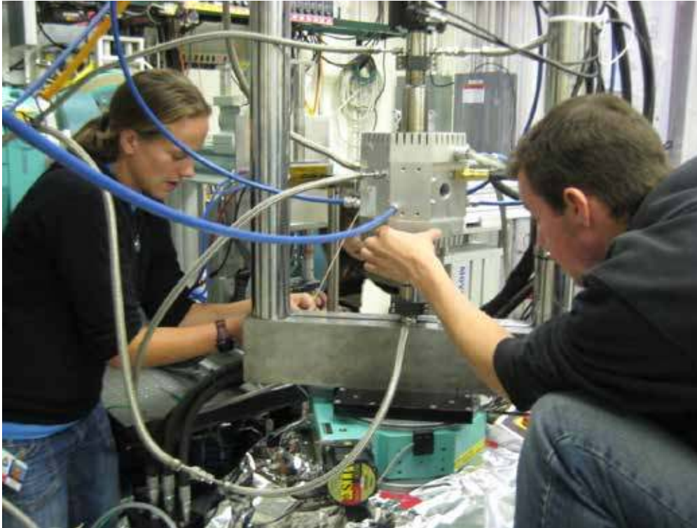
Assembling heater, grips and specimen at Argonne APS
