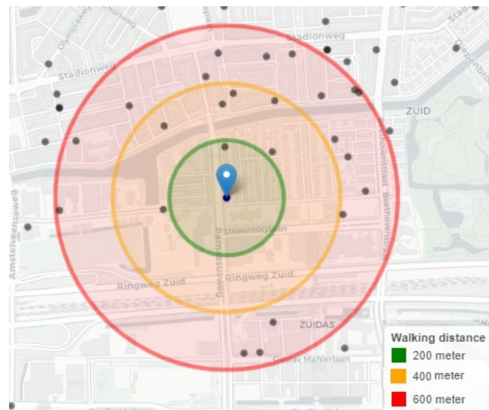
Figure 6.2 Charging stations within different ranges of walking distance in the Amsterdam-South area
