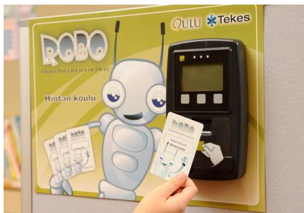
Figure 1. Pupil touches a reader device with a contactless smart card in order to log in the school.
