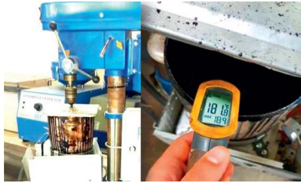
FIGURE 1: Mixing process of asphalt with SBS.
