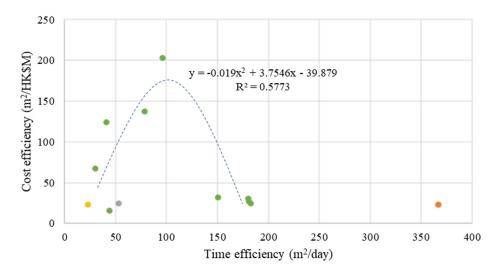
**Figure 7.** Measured time-efficiency and cost-efficiency. Notes: green dots–Projects A to I (modular QCs); yellow dot–Project J (conventional QC); orange dot–Project K (modular hospital); grey dot–Project L (conventional hospital).
