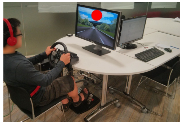
Figure 1. The setup of the experiment. Headphones, tactile belt and computer screen were used to deliver the multimodal signals.
