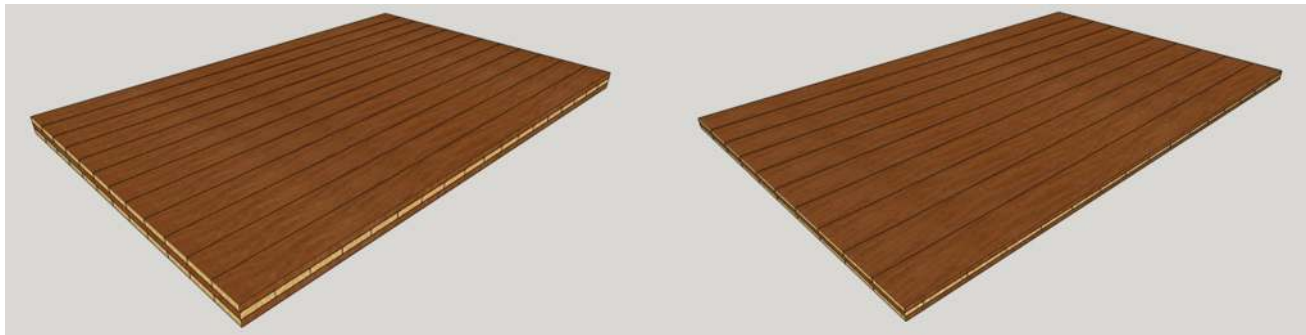
Fig. 1 CLT plates with 35/35/35 layup and 20/20/20 layup
