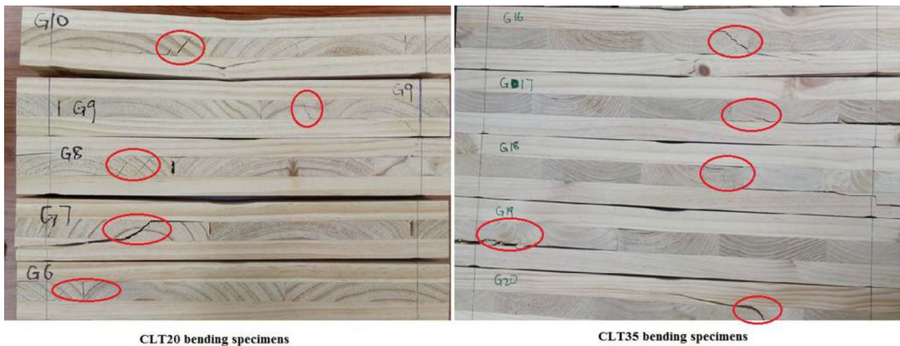
Fig. 4 Typical rolling shear failure modes observed in the bending specimens
