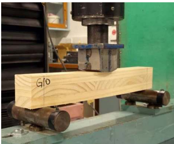
Fig. 2 Short-span bending test setup
