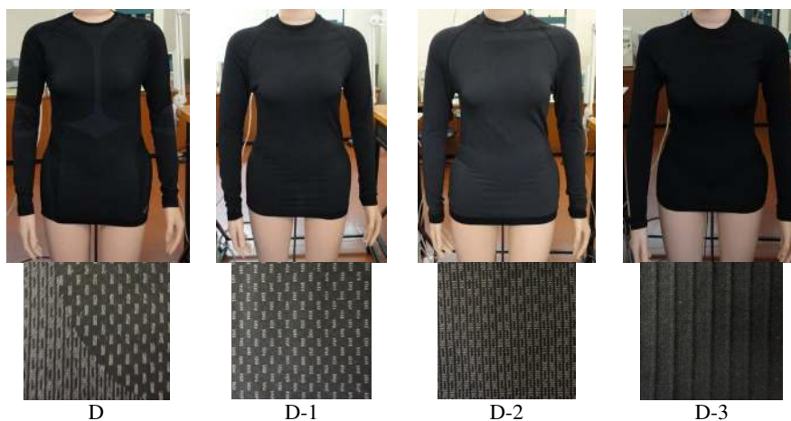
Figure 3. The type D shirts and views of the knitted structures
