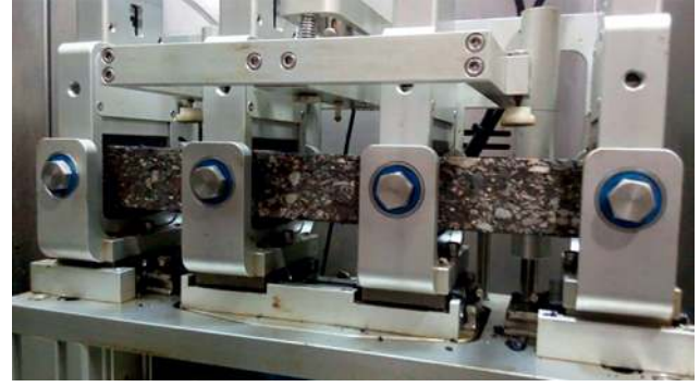
FIGURE 4: Four-point bending beam fatigue test machine.
