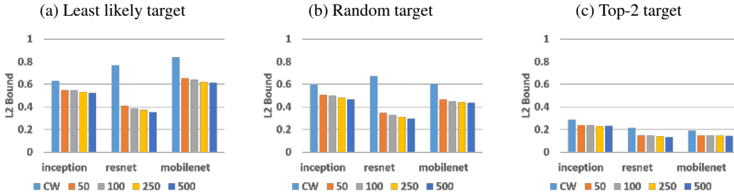
Figure 7: Comparison of the CLEVER score calculated by N_b = \{50, 100, 250, 500\} and the \ell_2 norm of adversarial distortion found by CW attack (CW) on 3 ImageNet models and 3 target types.
