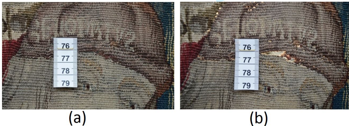
54 55 Figure 4: A close up from Figure 3; the effect of self-weight loading on damage propagation (a) just before 56 and (b) two weeks after unsupported tapestry display. Velcro fastener was used to hang the tapestry
