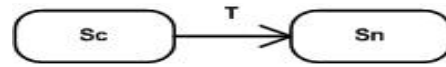
Figure 1. The STD Building Block (STD-BB) (Sc: moving forward, T: ApplyingBrakes, and Sn: Stop)
