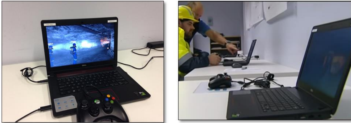
Figure 3-2: Semi-immersive desktop simulator (Desktop-VR) in Woonona, NSW (credits: Mines Rescue Pty Ltd)
