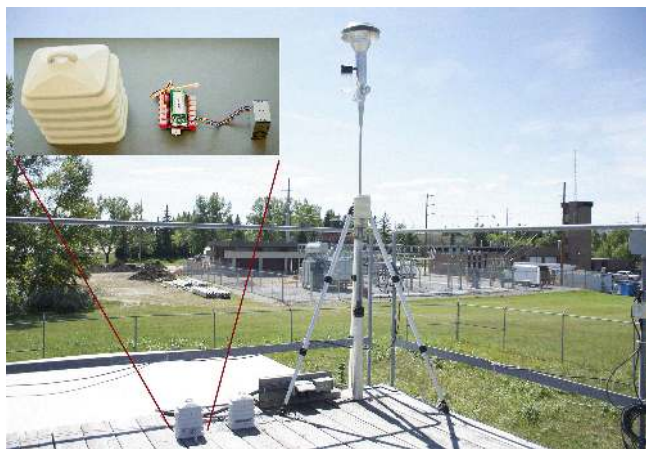
Figure 1. The low-cost sensor used in the study and the ambient inlet of the reference method – SHARP model 5030.
