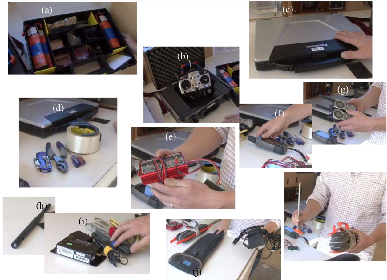
Figure 1.6: Ground Station Equipment: (a) backup box, (b) RC transmitter, (c) toughbook computer, (d) tools, (e) battery charger, (f) GPS receiver, (g) two way radios, (h) 900Mhz antenna, (i) 900Mhz modem, (j) tracker, (k) bungee
