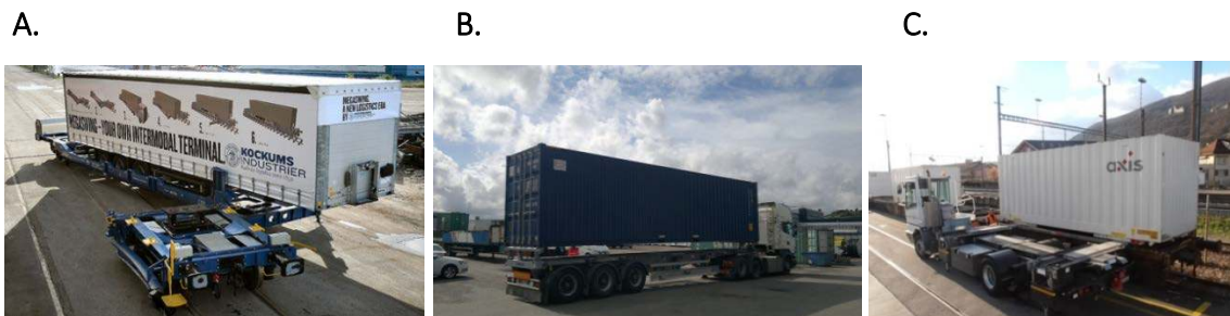
Figure 14.: (A.) Megaswing wagon (B.) CCT system (photo: Behzad Kordnejad, 2012) (C.) ContainerMover (photo: Behzad Kordnejad, 2014)
