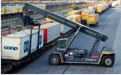
Figure 13. (A.) The Reach-stacker, a conventional technology used for transshipment of unit loads at intermodal terminals (source: Coop). (B.) The Light-combi concept (source: Axfood). (C.) JR Freight's "Effective & Speedy" system. (photo: Behzad Kordnejad, 2015)
