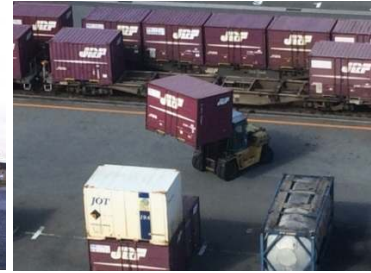
Figure 13. (A.) The Reach-stacker, a conventional technology used for transshipment of unit loads at intermodal terminals (source: Coop). (B.) The Light-combi concept (source: Axfood). (C.) JR Freight's "Effective & Speedy" system. (photo: Behzad Kordnejad, 2015)
