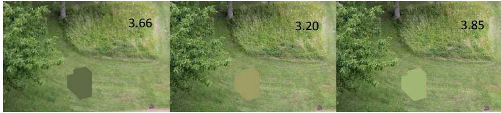
Figure 6. Synthetic CUBI on grass. The hue corresponds to the average hue of the grass background (61) and the saturation is 36% in all cases. The whiteness value is 42, 62 and 72, respectively.
