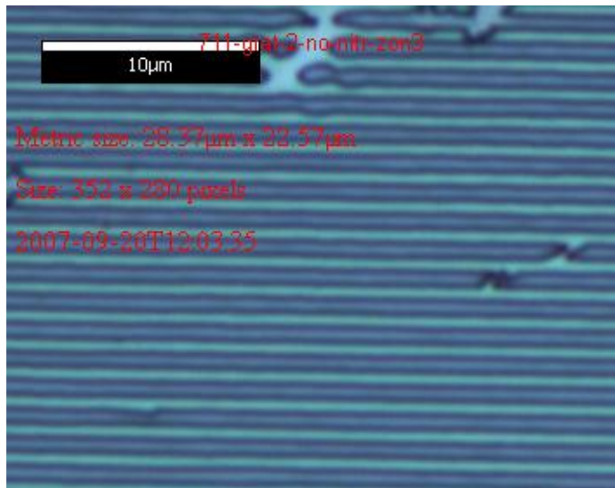
Figure 3: solar cell with 1D texturing without nitride antireflection.
