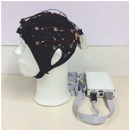
FIGURE 1: Channel layout of near-infrared spectroscopy (NIRS; Ch1–Ch9) and electroencephalography (EEG; (a)) and a headgear setup on a phantom head (b). Five sources (red circles, 1–5) and three detectors (green circles, 1–3) are located around Fp1, Fpz, and Fp2. Fourteen electrodes are located at Fz, F3, F4, F7, F8, C3, C4, T7, T8, Pz, P3, P4, P7, and P8. Reference and ground electrodes are located on TP9 and TP10, respectively.
