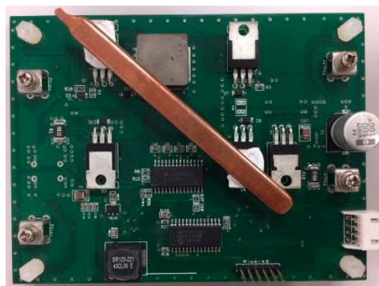
Figure 3. Front side of the direct current (DC)/DC optimizer with a heat pipe for a heat sink.
