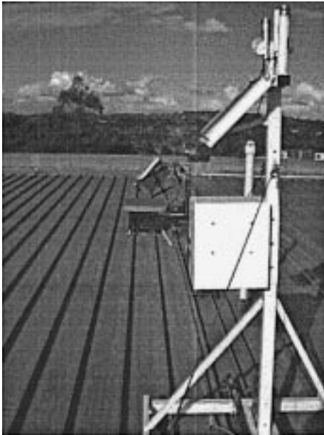
FIG. 1. Radiation measurement (datalogger in foreground) and sky image capture subsystem (power supply, camera, and stepper motor housing in the background).
