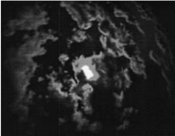
FIG. 5. Image 2: 256 Grayscale 200 \times 256 pixel image of cloudy sky (1041 LT 11 Sep 1997). This corresponds to data point 15 of Fig. 8. Disk obscured and 79% cloud cover in FOV.
