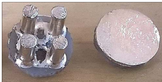
Figure 1: Gold coated dry multipin electrode for electroencephalogram recording through the hairs and dry flat electrode for electrocardiogram or forehead-electroencephalogram recording. The electrode's base had a diameter of about 11 mm
