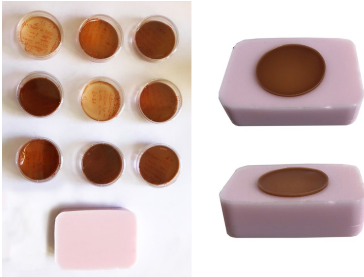
Figure 9 Images of the components to the multi-layer phantom constructs developed to emulate pigmented nevi at multiple thicknesses. Thin layer samples fabricated with the same concentrations of absorber and scatterer, but at multiple thicknesses based on the volume used (left). Assembly of two-layer construct with coffee phantom layer placed on top of the pink (dermal) phantom (right). All SFDS measurements were collected from 3 central locations within the coffee phantom disk.
