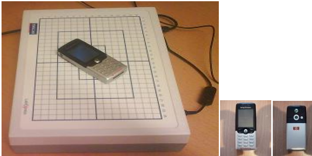
Figure 15 DUT (7) phones in 8 positions
