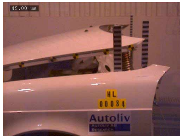
Figure 4. Bonnet with protection system in activated (lifted) position.
