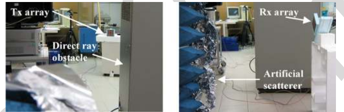
Fig. 10. MIMO measuring environment: (a) transmitting array; (b) receiving array.
