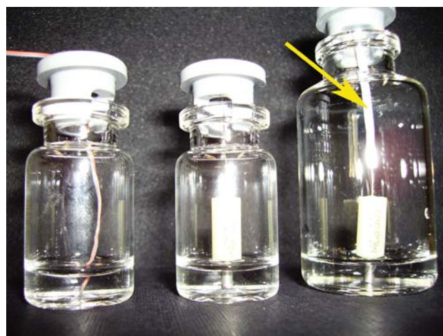
Fig. 2. Correct placement (bottom center) of a thermocouple (left) and two TEMPRIS sensors (5 mL and 20 mL vial, right). The TEMPRIS sensor can easily be fixed in this position by a small teflon tube in the stopper
